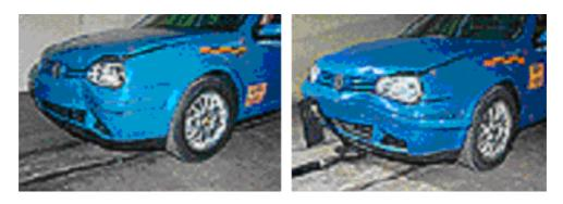
VW Golf IV—Identical deformations following AZT crash repair test on passenger vehicle in original condition (above) and following correct repairs (below).
