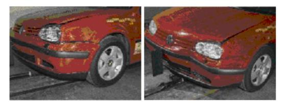
After the AZT crash repair test: Identical deformation of the vehicle, original (above) and after professional repair (below). Photo: Allianz Versicherung
